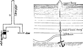
to which was fixed the large buoy floating on the surface with plenty of slack chain to allow for rise and fall of tide, and this buoy also marks the position of the flexible pipe.
